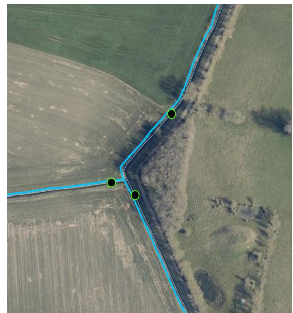
Figure 8 – The triangle format on of stations at the confluence of two streams.
